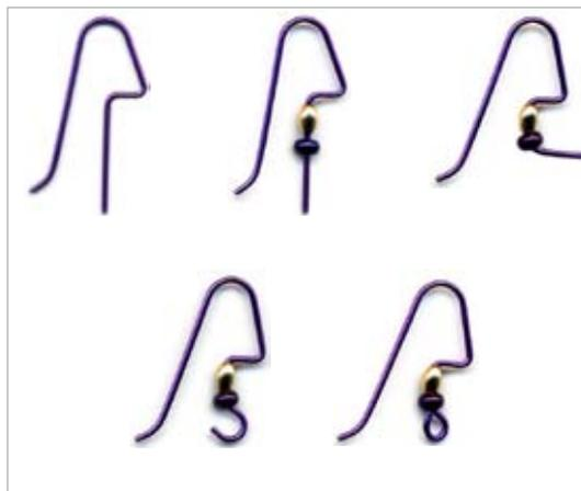
Anodized niobium ear-hooks, such as these, are available in a range of beautiful colours that can be damaged by rough handling, so when forming loops, cover the jaws of your pliers with clear adhesive tape to protect the colour finish.
